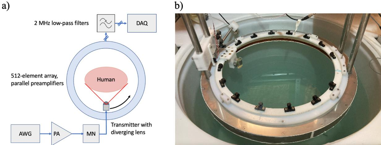
Figure 1. a) System diagram. AWG: arbitrary waveform generator; PA: power amplifier; MN: matching network; DAQ: data acquisition module. b) System photograph.
